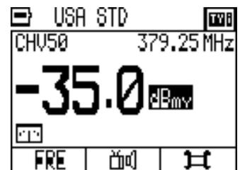
The unit will display the audio carrier frequency, the signal strength and play the audio.
