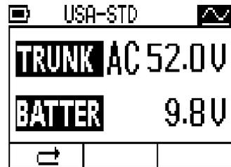
The meter will automatically identify "AC" or "DC" of the trunk voltage, and display on the screen. The battery voltage also display on the bottom.
